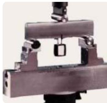
**Fixture for 3-point and 4-point flexure testing of beams**
