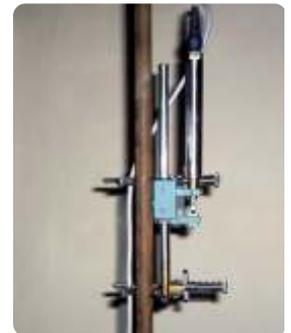
**Electronic Extensometer (LVDT) based**
