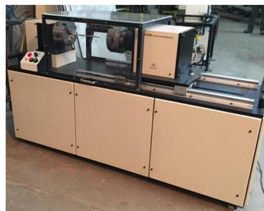
TSTM is a line of microprocessor controlled motorized machines designed to automate, simplify and standardize the strength different types Torsion Springs and different specimen both in clockwise and counterclockwise direction. Electronics Torque Transducers are used measure the torque and optical encoders to measure angle of rotation accurately.
